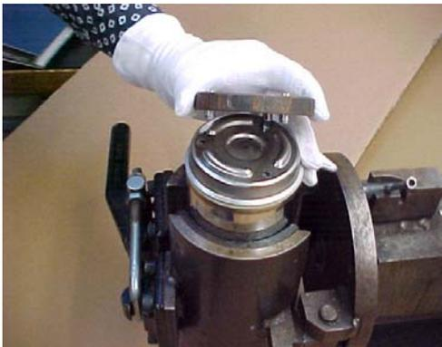
2. Assemble Anode with supplied screws each one separately against bottom cover of the Motor
