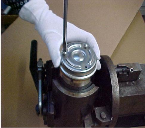
1. Remove one screw and washer at a time from the bottom end bell cover of the Motor
